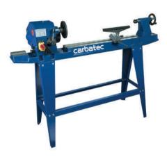
Perfect for the beginning or budget-conscious woodturner. The speed is variable via a split pulley system that allows the spindle to run between 500 to 2000 rpm. While the motor is running, turn the handle, allowing the pulleys to separate giving a different belt ratio, therefore changing the
