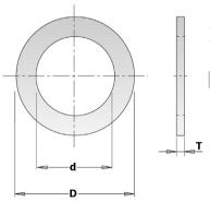
Used to insert into the arbor of a saw blade to match the smaller saw arbor.
