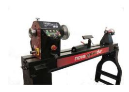
Nova introduce their new GALAXI DVR lathe. The DVR (Digital Variable Reluctance) motor is computer controlled, there are no belts, no brushes or anything that wears, providing the highest torque at the slowest speed down to 100 rpm, all the way through to 5000 rpm. The bed is precision ground allowing for the headstock, tailstock and banjo to be moved along
