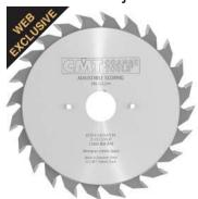
Used on a vertical or horizontal panel saw to prevent chip out on laminate materials. Smaller in size that the main blade, it spins in the opposite direction to that of the main blade, and cut a channel slightly wider than the main blade, but not wide enough to be noticeable when edge tape is applied. Shims placed between the two split blades to match the main blade.
