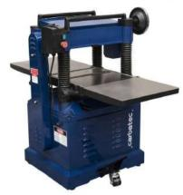
The Carbatec TH-381C thicknesser is literally stacked with features and will be a welcome addition in any workshop big or small. Features a powerful 3HP motor, a three knife cutterhead, serrated infeed roller, polyurethane outfeed roller, anti-kickback fingers, adjustable bed rollers and a front-mounted Magnetic Starter NVR switch.
