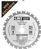
Featuring alternate top bevel ground teeth, narrow kerf, low number of teeth and a 20 deg, hook angle, this ripping blade is ideal for glue line rips in hard and soft woods.
