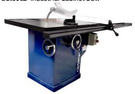
An excellent machine for the home enthusiast, trade user or discerning . The large, precision ground cast iron table surface provides a solid footing for real work to be accomplished. An industrial style T-fence is fully adjustable and can be calibrated to ensure reliable and accurate cuts. To provide safety and visibility,the machine includes dust extraction ports at the top of the blade guard and at the base of the machine, collecting dust at the source giving you a clear view of your work.
