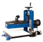
This machine is ideal for finish sanding on any timber, but excels on curlygrained, quilted or birdseye timber. A massive 125mm throat depth allows you to do larger pieces. Couple that with a powerful 1hp motor induction motor and you have a winning combination. A dust extractor is a must with this machine, and we recommend at least a 2HP (or any extractor in excess of 1000CFM). This greatly increase the effectiveness of your machine and
