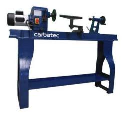
A tremendous new lathe model with all the features of a larger professional quality lathe. The speed is variable via a split pulley system that allows the spindle to run between 500 to 2000 rpm. While the motor is running, turn the handle, allowing the pulleys to separate giving a different belt ratio,
