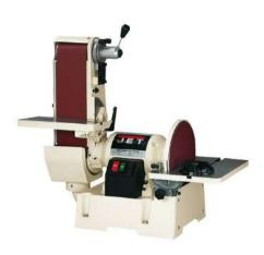
The ideal belt and disc sander for all workshops from novices to professionals. The JET JSG-6DC Sander boasts a 12" disc and a 6" wide belt powered by a 1.5 HP motor. Tracking is easy via the dual thumbscrews, with a quick release lever to release the belts for easy removal.
